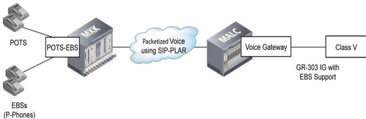
Figure 170: POTS-EBS card supports packet voice
